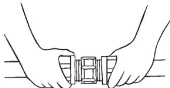
The full hydraulic seal is achieved when the pipe passes through the seal ring. Nut tightening is only to achieve pull-out resistance – the hydraulic seal is automatically created when the pipe is pushed past the seal ring.
