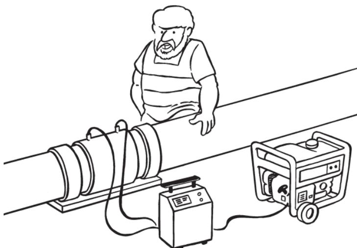
You'll need a good power source. If you don't have one fire up your genny...Remember... check the gas tank, make sure it's full and ensure all the cords that you plan to use are in good health. The EF control unit should be checked to see that it is compatible with the fittings that you plan to fuse. Connect the cables to your fitting and begin the fusion process.
