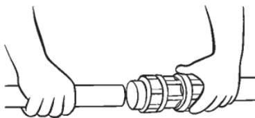
4. Firmly hand tighten nut. Use a wrench for a further half turn past hand tight for final tightening of fittings diameters 40mm and greater.
