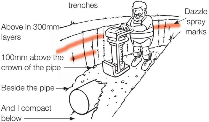
Compacted granular bedding/aggregate surrounds the pipe and up to a minimum 100mm above the pipe. Then I use selected ordinary backfill. I compact with my machine below, beside and above the pipe in layers of 300mm until I get to the top surface.
