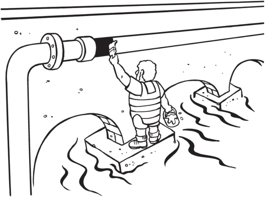
Hey, black pipes are the best to use outdoors cos black reflects the ultra violet rays better. U.V. attacks coloured PE pipe real quick! If you need to use striped or colour skin pipe for some reason, paint 'em with a light coloured acrylic paint... The light colour paint will reflect the heat in those hot summer months.
