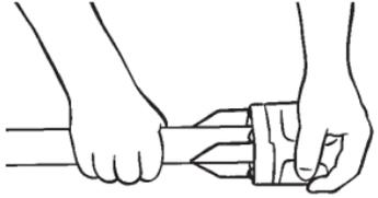
The manufacturer strongly recommends the use of PTFE tape in threaded connections (don't use hemp), I always use it! But don't put too much on – three wraps should do.
