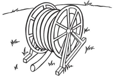
There can be a lot of stored energy in coiled PE pipe. Make sure the pipe-end is strapped down tight and the brake is on securely! Here's another way to do it... 125mm PE pipe made into coils then placed onto a pipe dispensing trailer.
