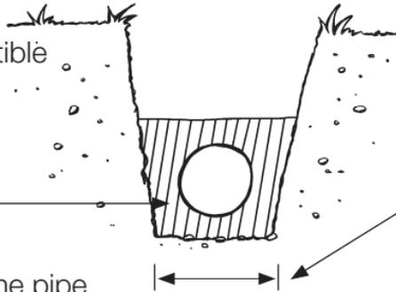
Pipe size – plus 300mm (This saves backfill material as well!)
