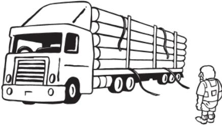
Check the pipe when you get ‘em on site. Unload carefully. **Never** tip ‘em off. When ya unstrap the load keep **way back** from it cos PE Pipe is as slippery **as an old eel!**
