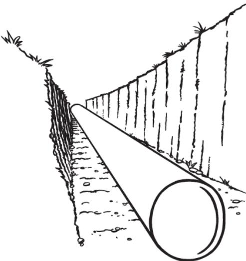
When ya' in the rural blocks take the **FFP** approach... but use your common sense... big boulders and organic material (lumps of turf) don't work as bedding, get 'em out. Use loose selected as dug material in the backfill zones, remove the big boulders as they could damage any plastic pipe!
