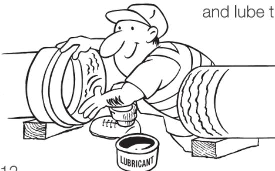
I get Willy to line up the spigot into the socket. Willy never drops the lubed spigot onto the ground cos the bedding sticks to it which will make the seal leak if not cleaned properly...
