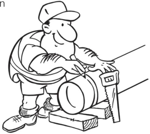
I measure the pipe socket inside and subtract 5mm to make it shorter. This is the **witness mark** measurement. The witness mark should be **just visible** once installed.
