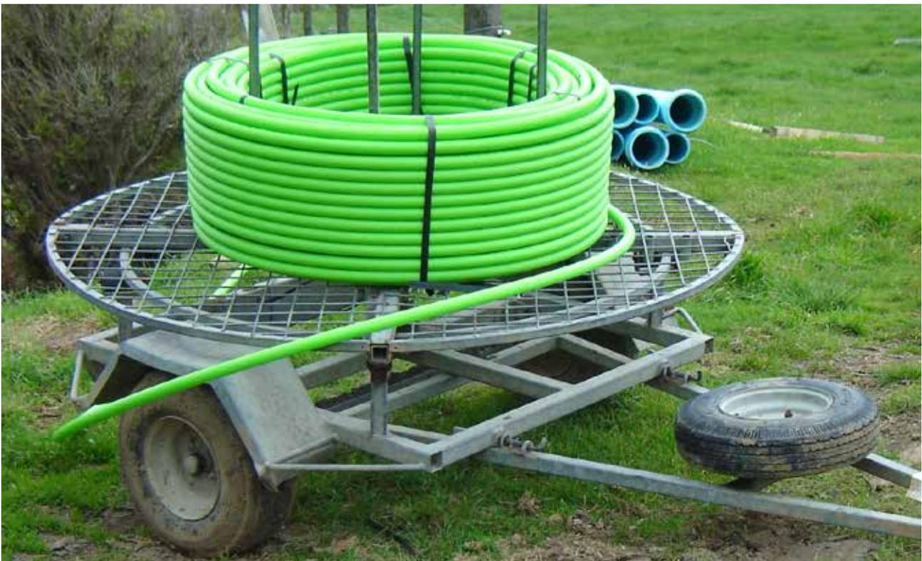
Image 4. Small Free Standing Coil on a reel dispensing trailer.
