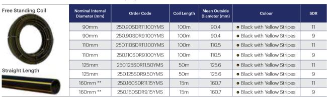
Iplex strongly recommend that mechanical straightening and mechanical re-rounding equipment be used when installing DN160 pipe. Manufactured to AS/NZS 4130 Series 1\*\* Straight Lengths
