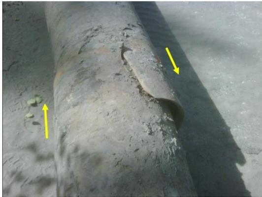
*Figure IX - Compressed joint movement in CLS water main, Christchurch*
