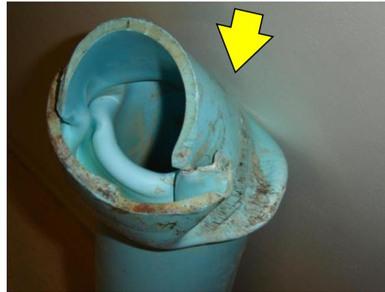
*Figure XII - Ductile axial compression folding in PVC-U pipe, Gayhurst Road overbridge*
