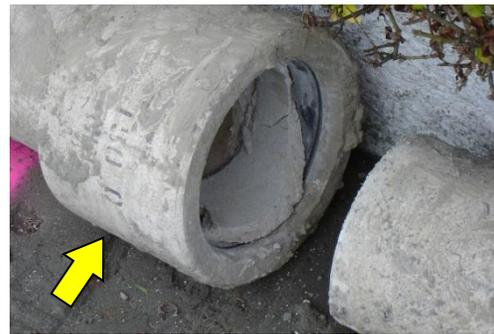
Figure VIII – Shear effects in AC pipe joint, Jollie Street, Kaiapoi, with tangential alignment to the Darfield epicenter, 2010
